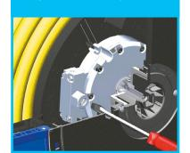
Overrun protection on spring prevents spring damage on drum overrun
